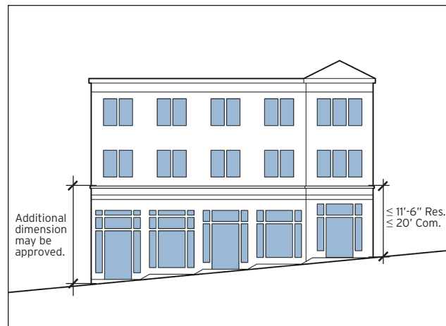
Figure 860-09: Additional First Story Dimension
